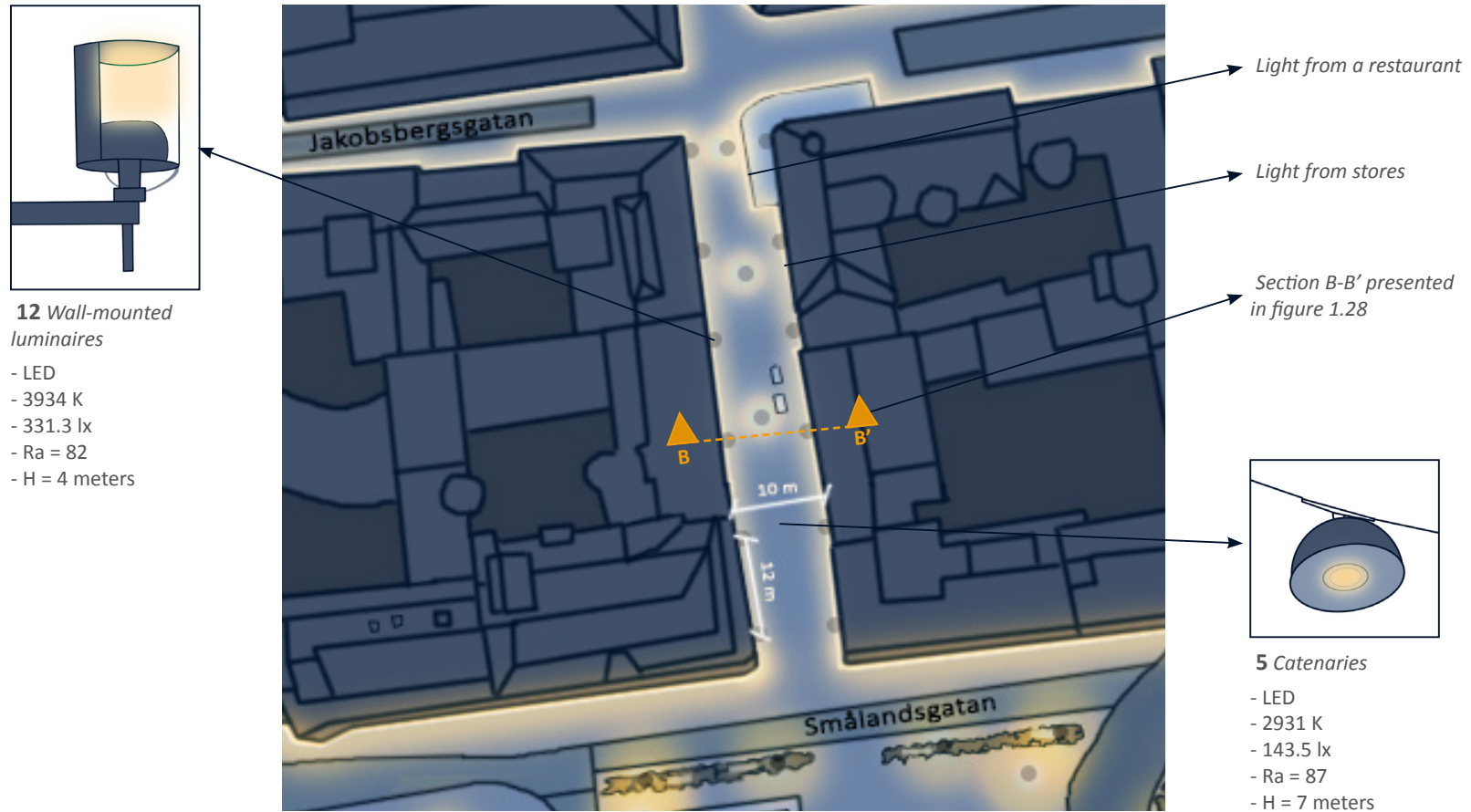
Figure 1.29 Biblioteksgatan: Light' position, lighting levels and color - Plan of the current lighting layout - The measurements of lighting levels, color temperature and color rendering index were taken on the floor level below the urban fixtures with a CL-500A illuminance spectrophotometer | Scheme: Done by the author following the methodology of "Lighting Detectives: Newsletter vol.86"
