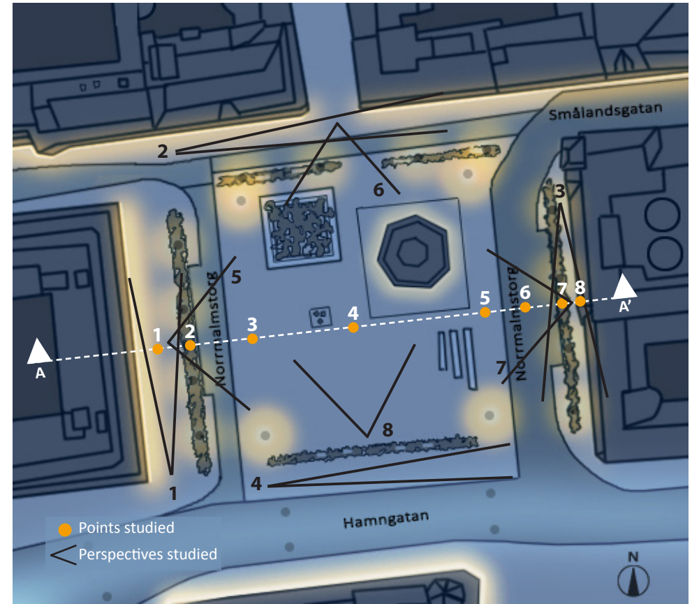
Figure 1.12 Normalmstorg : Evidence studied to structure the author’s quantitative measurements - The measurements of the lighting levels were taken in eight (8) different points by using a CL-500A illuminance spectrophotometer Konica Minolta - The HDR images to study the perception of a person’s face were taken in the same eight (8) points by using the app Aftab Luminance - The HDR images to study the lighting distribution were taken from eight (8) different points | Scheme: Author
