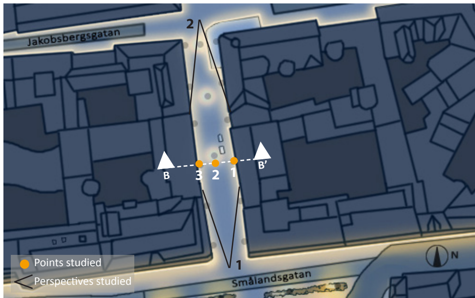
Figure 1.11 Biblioteksgatan : Evidence studied to structure the author’s quantitative measurements - The measurements of the lighting levels were taken in three (3) different points by using a CL-500A illuminance spectrophotometer Konica Minolta - The HDR images to study the perception of a person’s face were taken in the same three (3) points by using the app Aftab Luminance - The HDR images to study the lighting distribution were taken from two (2) different points | Scheme: Author
